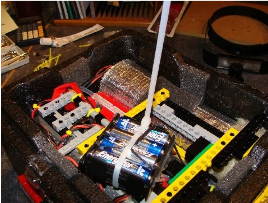
Fig. 10 : Secure the batteries from slipping out of the holder with the help of a cable binder.
