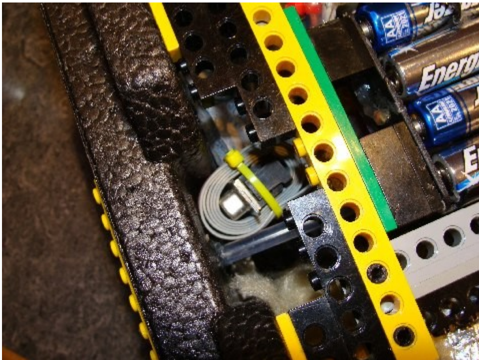
Fig. 15 : This RS232 cable should be unrolled and connected to a PC. (The battery block needs to be removed from its location in order to reach the cable.)
