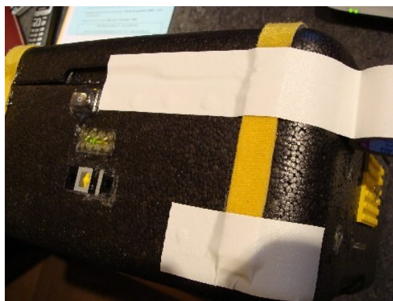
Fig. 14 : The Velcro fasteners need to be secured and the slit between the main body of the container and the cover needs to be closed with adhesive tape.
