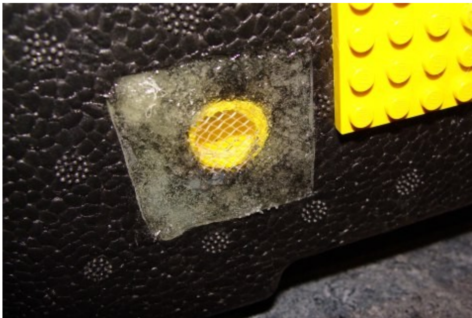
Fig. 4: The air inlet for the ozone sensor with protective Mosquito net on the top of LUXPAK
