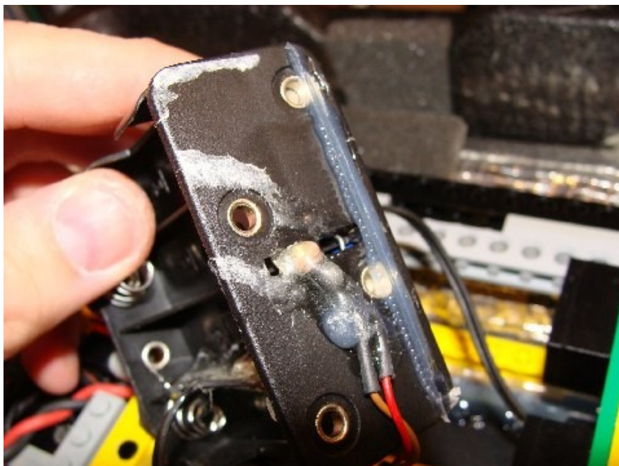
Fig. 9 : The thermistor has been glued to the side of the battery holder.
