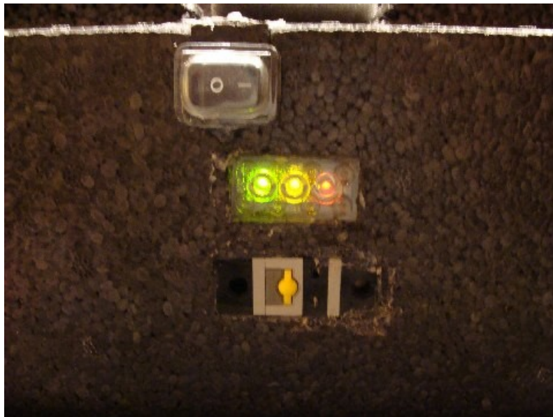
Fig. 6 : LUXPAK's main switch starts the whole engine except the datalogger and the ozone tube heater. If LUXPAK is ready, the yellow LED goes on. Once the datalogger is running, the green LED also shines. Beneath the transparent LED block is visible and finally the RCX button that has to be released before launch in order to activate all vital flight functions.
