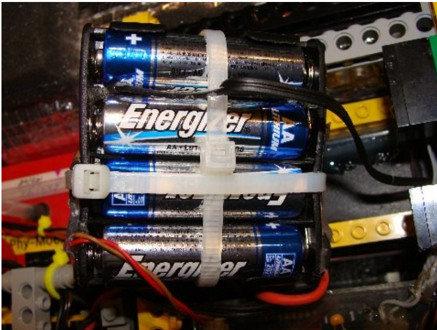
Fig. 11 : The second binder should cross the first one and should not be forced too much. On this picture the battery holder is already squeezed, which could damage the holder. The ground operators must be very cautious here.
