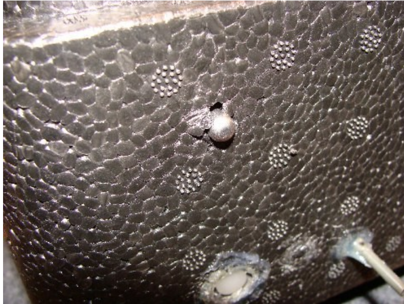
Fig. 5: The air outlet stud from the ozone sensor system can be seen on LUXPAK's bottom (right picture corner). The ESR light sensor is visible and in the upper region of the picture also the PT100 temperature sensor.
