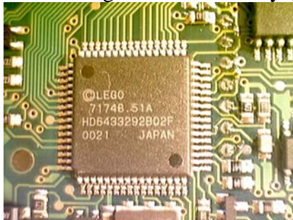
Picture 3: The RCX H8 micro-controller in its FP-64 package
