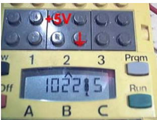
Picture 1: Paradoxically “unpowered” sensor ports present a voltage of 5V.
