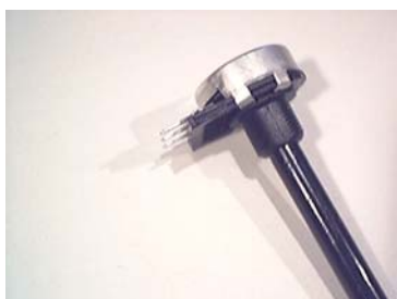
Pictures 4 & 5: Example of a resistive sensor : a potentiometer measuring angles that may easily be hidden into a LEGO brick and equipped with a gear. Unfortunately the original LEGO connector must be cut and soldered to the pins of the variable resistor.
