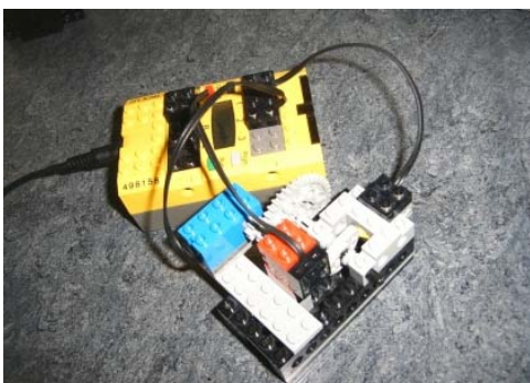
Pictures 33 & 34: The test assembly for the converted angle-sensor experiment. Note the use of the eccentric cam.
