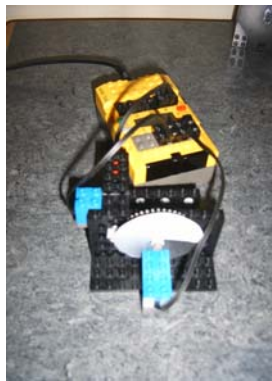
Pictures 11 & 12: The new gradual encoder with the test-bench. i
