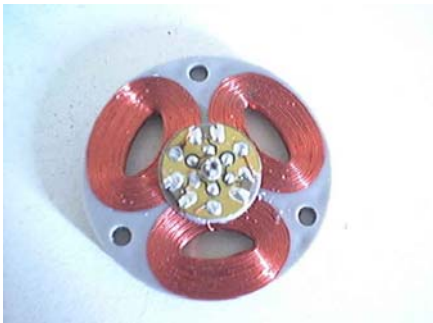
Picture 30: A LEGO motor anchor composed of three coils and 6 connections. The motor brushes slip over the shaft and realize the polarity-reversing of the induced current.
