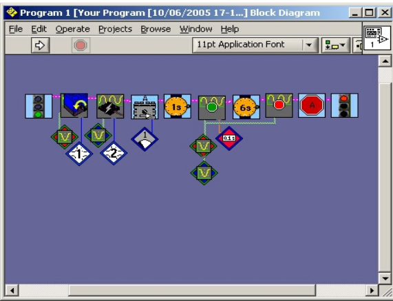
Picture 21: This program first configures the datalogging for the two sensors, starts the motor at lowest power level, waits a power-up second and logs the data for 6 seconds.
