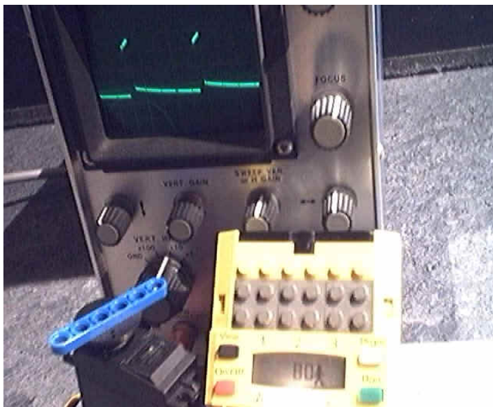
Picture 23: RC-servo motors are controlled with a short 30-50Hz pulse. The information about the servo-position is transported by the pulse width.
